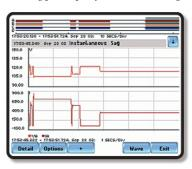
to events can be determined so that corrective measures can be implemented. The PowerXplorer has a built-in event characterizer that directly supports troubleshooting and the gathering of survey data—for improving power quality and equipment reliability, as well as for matching the requirements and susceptibilities of that equipment to the incoming supply.
